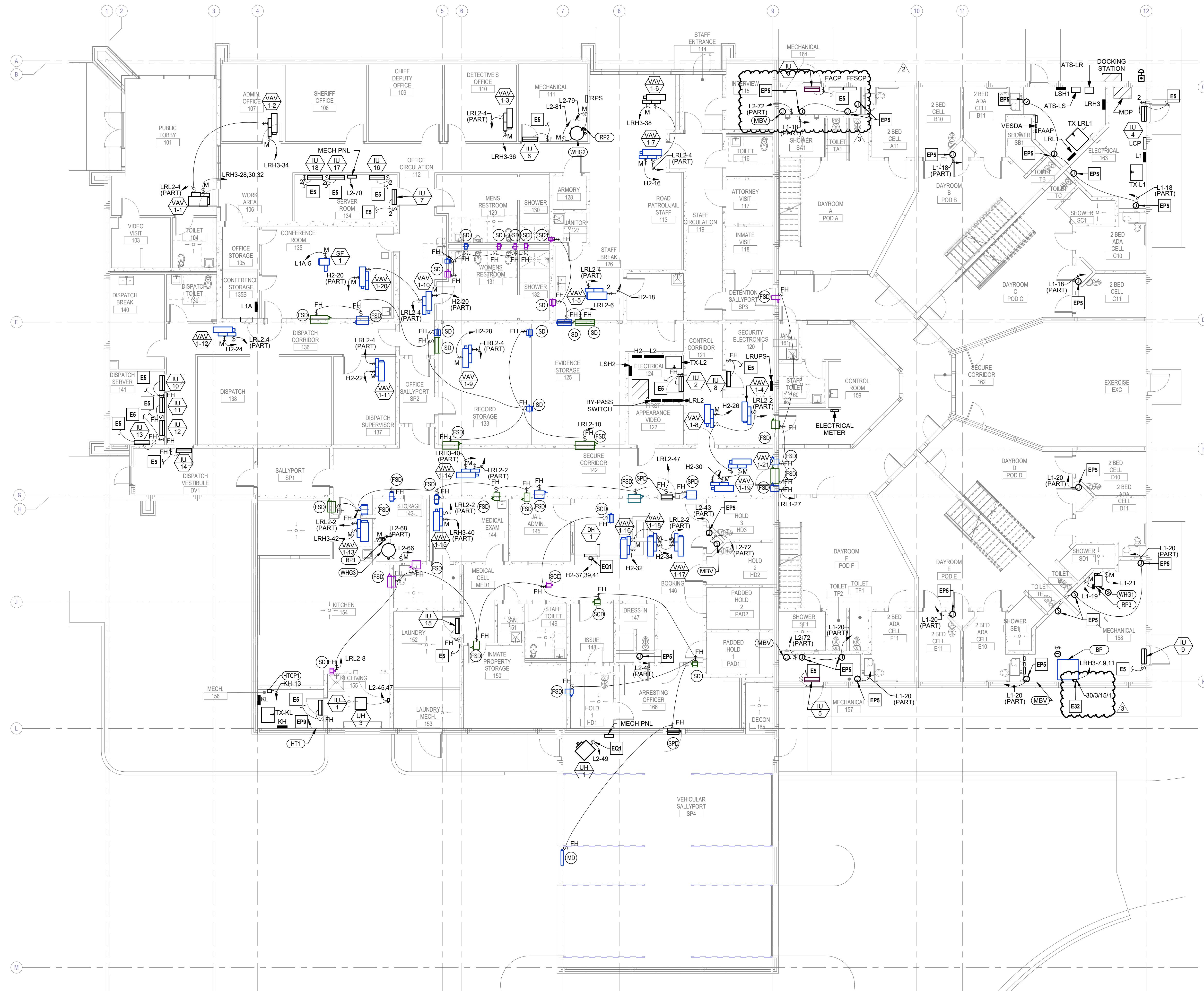
1 EQUIPMENT CONNECTION FIRST FLOOR PLAN - OVERALL 1/8" = 1'-0"
